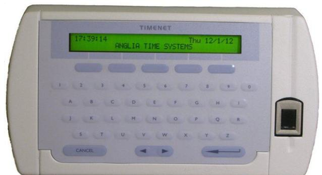
Biometric terminal using finger-print
