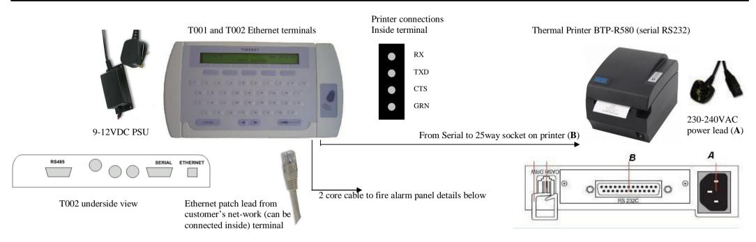
Connection to terminal from PC or Workstation via TCP/IP-UDP (RJ45 socket) Port5007 or RS232 Data cable 2 - twisted pair screened
